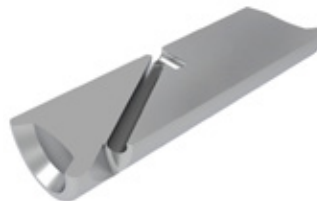
Bearing lubrication passages via radial or angled holes
