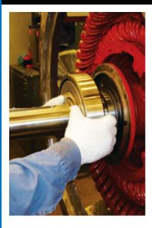
Koyo's 3NC Hybrid Ceramic Ball Bearings are filled with Exxon Polyrex<sup>®</sup> EM Grease
