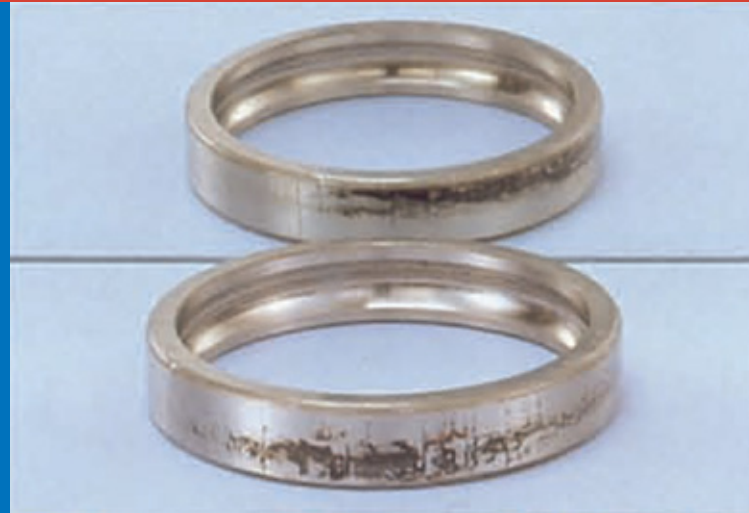
Phenomenon: Symmetrical Fretting on Upper and Lower Sides of Raceway
