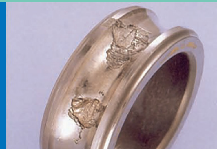
Phenomenon: Flaking at Intervals on Ball Pitch Cause: Indentations Caused by Impact Load Develop into Flaking
