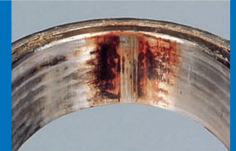
Phenomenon: Scuffing on Bore Surface Cause: Diagonal Assembly or Foreign Matter on Fitting Surface
