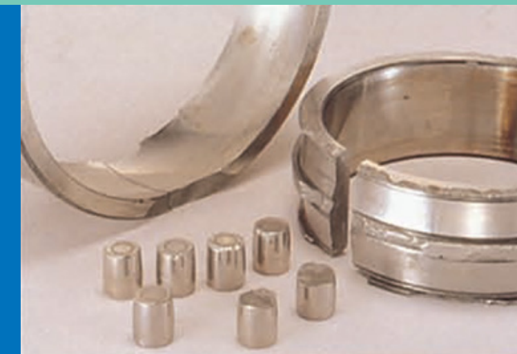
Phenomenon: Cracks and Chips on Inner and Outer Rings and Rollers (Left) / Seizure Caused by Chips on Ribs (Right)
