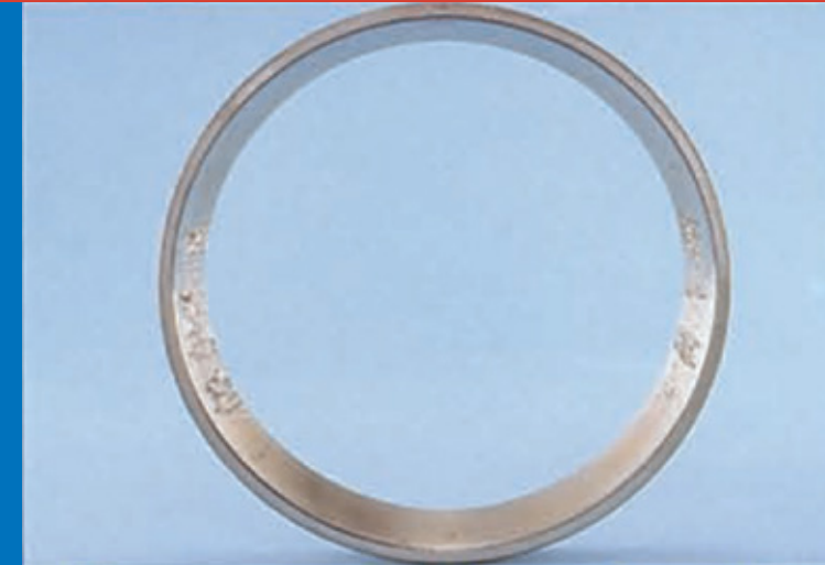
Phenomenon: Flaking on Opposite Faces of Raceway
