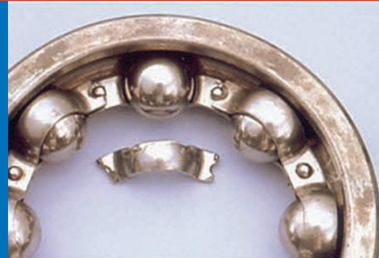
Phenomenon: Broken Retainer
