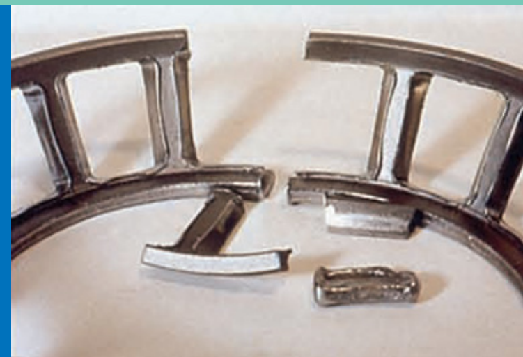
Phenomenon: Broken Retainer
