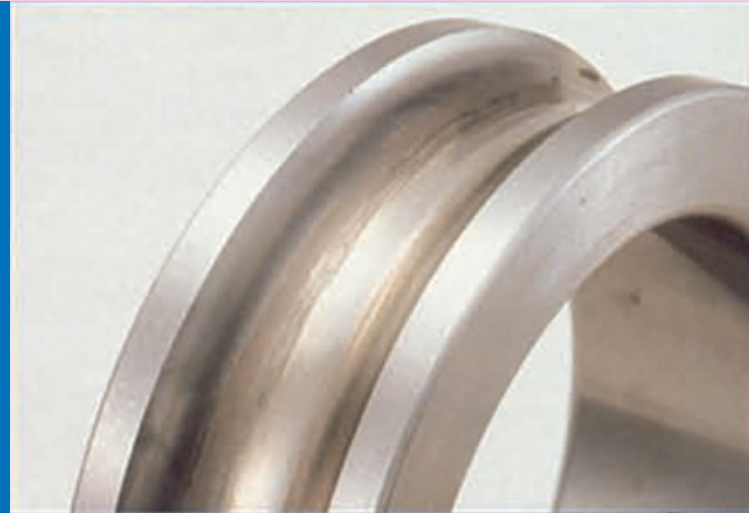
Phenomenon: Smearing on Raceway
