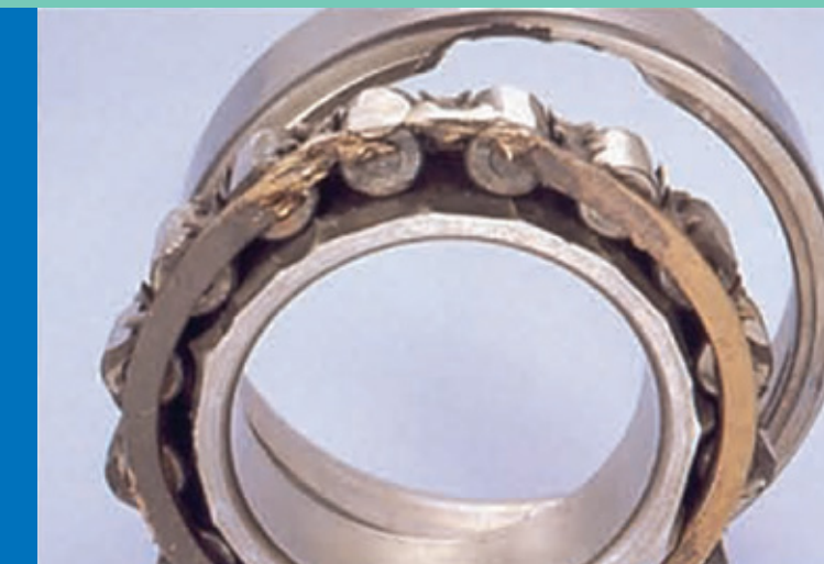
Phenomenon: Cracks and Chips on Inner and Outer Rings and Rollers (Left) / Seizure Caused by Chips on Ribs (Right)
