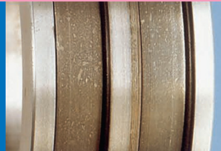
Phenomenon: Indentations on Raceway
