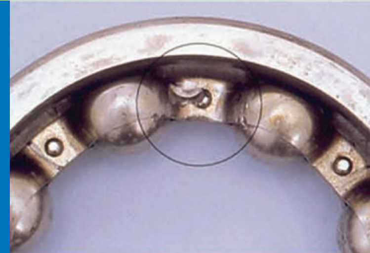
Phenomenon: Dents on Retainer
