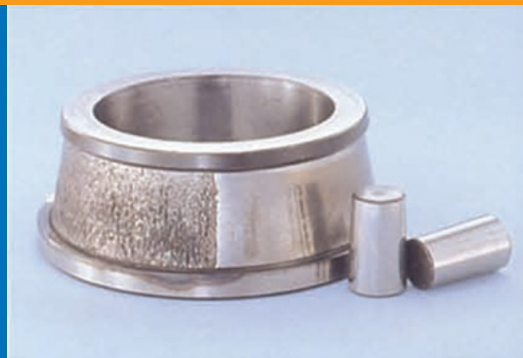
Phenomenon: Flaking Generated Around Half the Raceway
