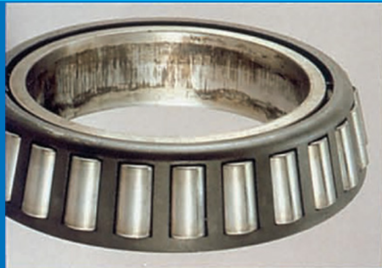
Phenomenon: Fretting Corrosion (Left)
