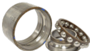
INBOARD RACEWAYS - Good condition
