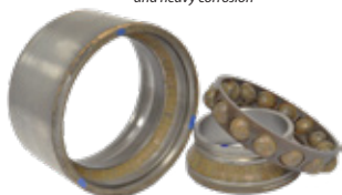
INBOARD RACEWAYS & BALLS - Heavy corrosion
