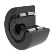
RITETRAK™ track rollers are sealed to keep contaminants such as dust and dirt out, while retaining lubrication. In tandem with an increased grease capacity, this allows for maintenance-free operation without re-lubrication over the life of the bearing. Featuring a double row of larger-diameter cylindrical rollers within the same envelope dimensions, RITETRAK™ bearings last up to 4x longer and are a direct replacement over standard needle roller designs.
