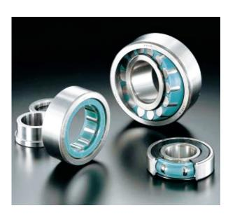
Koyo Solpack™ bearings come pre-filled with a solid polymeric lubricant. Solpack bearings are available as deep groove ball bearings and spherical roller bearings (with OD of 200 mm or less). Typical applications where Solpack bearings are used include food processing lines such as canning or pickling lines, washing facilities, or plating lines.
